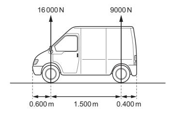
The van is  $2.50\,\mathrm{m}$  long with the wheels at a distance of  $0.600\,\mathrm{m}$  from the front of the van and  $0.400\,\mathrm{m}$  from the rear of the van.
