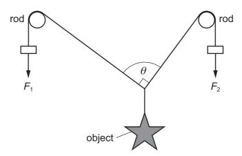
The object is held in equilibrium by the forces  $F_1$  and  $F_2$ . The object weighs 10 N. There is negligible friction between the rods and cords. Angle  $\theta$  is 90°.
